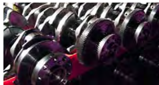
Henkel's experience in retaining cylindrical components using shrink bonding helped Ford to engineer a bonded solution
