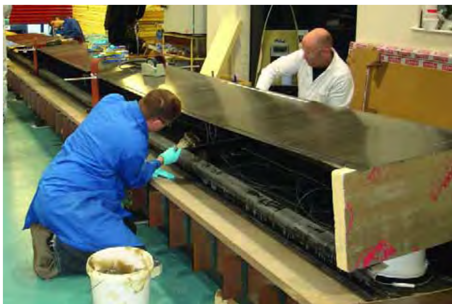
Application of Crystic Crestomer adhesive to spar caps and upper skin
