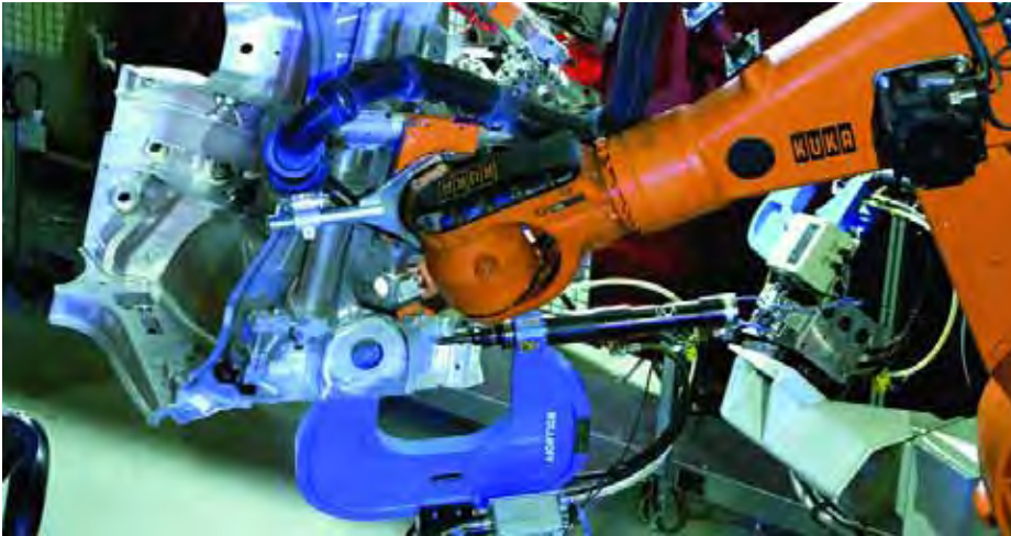
Automotive body assembly with Rivset within an automated robot system
