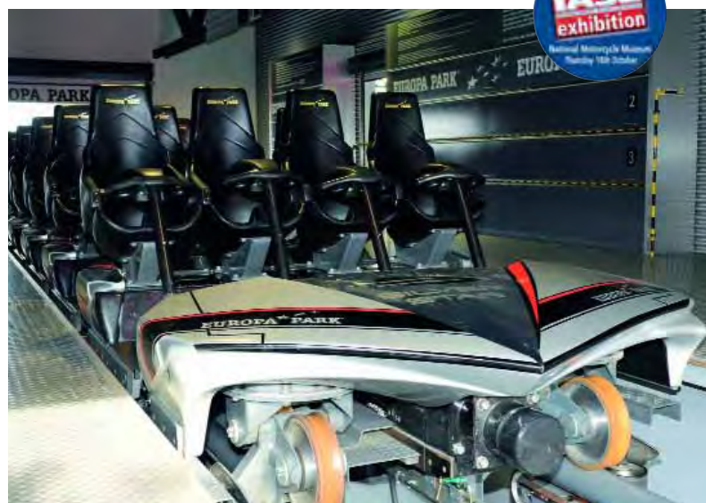
The all-important safety bars are secured with a threadlocker after maintenance inspections
