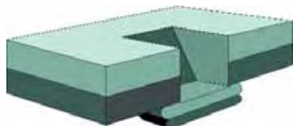
A rectangular joint is formed by lancing the metals on two sides
