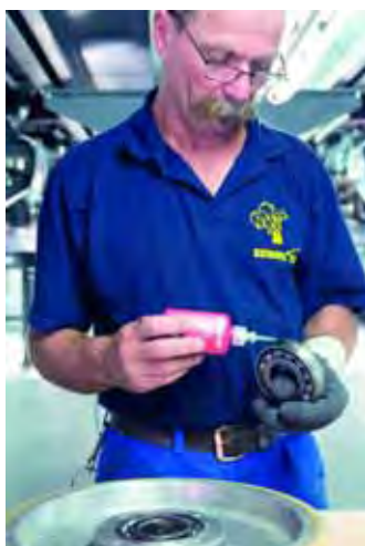
Retaining the ball bearing casing with Loctite 638
